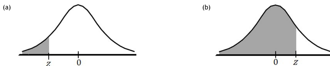
Fig. 2. The shaded region in the graph represents the table entry for (a) negative z-scores and (b) positive z-scores.
