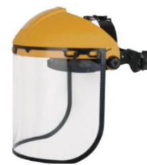
Figure 2. Face shield class 6 fit snugly (adjustable) along the brows to the corners of the eyes, extends to the ears, the crown, and past the chin, are an alternative to goggles, and protect from splashes and impact.
