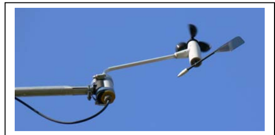
Figure 8: Wind speed sensors like this one used by the authors are not common, but it should be used along with air temperatures to decide if wind machines should be turned on/off, or if winds are favourable for operation.
