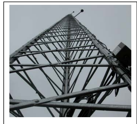
Figure 7: A 20 m (66 ft) tower monitors air temperatures from ground level to the top, plus wind speeds within the influence of a wind machine
