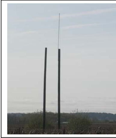
Figure 6: Growers use a tall pole with sensors top/bottom for monitoring ground and inversion level air temperatures
